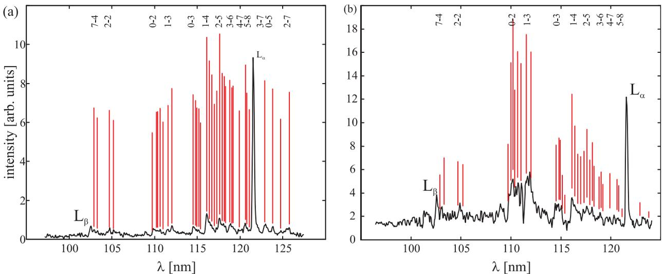
**Figure 4.** Examples of spectra of the atomic hydrogen  $L_\alpha$  and  $L_\beta$  transitions and rotational–vibrational transition of molecular hydrogen belonging to the Werner band system.
