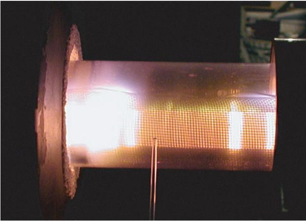
**Figure 2.** Photograph of the type III cell. Bluish-white light can be seen at positions up to a few centimetres outside of the oven (left) and the brass insulator (right).
