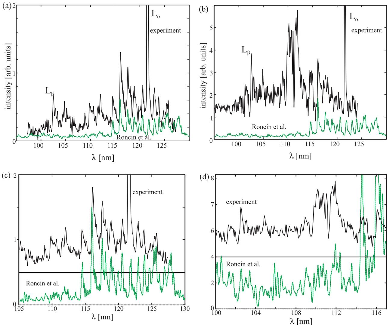
**Figure 5.** The measured molecular hydrogen spectra of figures 4(a) and (b) are compared with synthetic emission spectrum (intensity-scaled) after [18] in (a), (c) and (b), (d), respectively.
