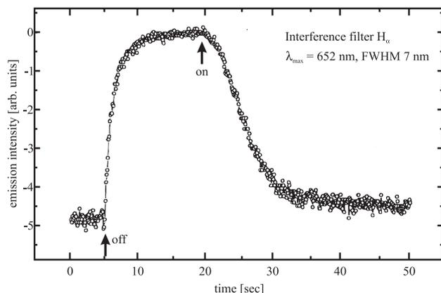
**Figure 1.** Emission of the cell as a function of time while the filament current was turned off and on. The plasma decay with no electric field present followed the decay of atomic hydrogen from the filament dissociator. Upon restoration of the filament temperature, dissociation and the plasmas resumed.
