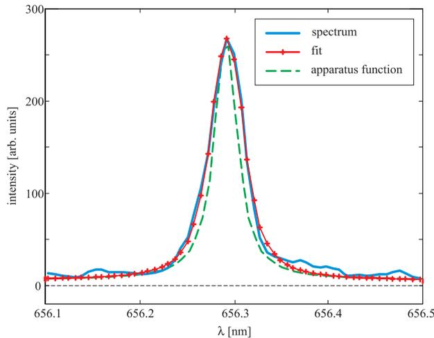
**Figure 3.**  $H_\alpha$  emission measured in the second order together with the best fit and the apparatus function.
