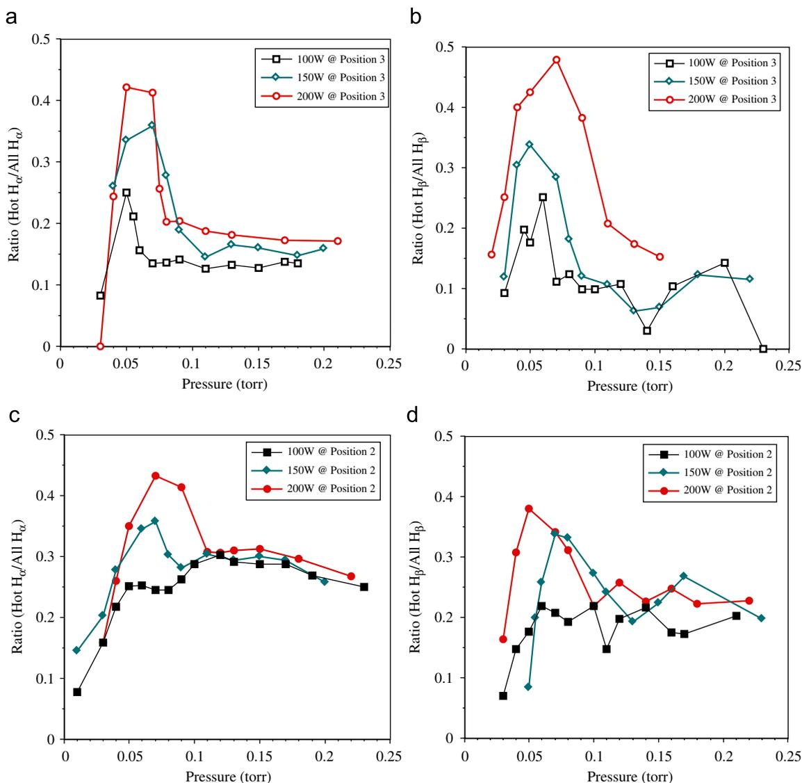
**Fig. 5 – ‘Hot’ hydrogen between 10% and 45% of all atomic hydrogen. (a) and (b) At a position 15 cm from the electrode the fraction hot hydrogen varies as a function of pressure, and power to a lesser extent. Virtually identical trends are observed from the  $H_{\alpha}$  and  $H_{\beta}$  data. (c) and (d) The trends in fraction hot hydrogen as a function of pressure and power are virtually identical between the plates and at 14 cm from the plates.**
