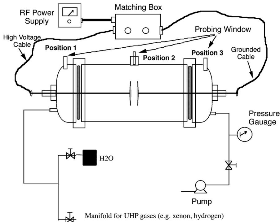
**Fig. 1 – Cylindrical RF Plasma System. Length: 35 cm, radius 14 cm. Positions 1 and 3 are 15 cm from the center. Note, most data collected at Position 2 (high field) and at Position 3 ('grounded electrode' and gas exit position).**
