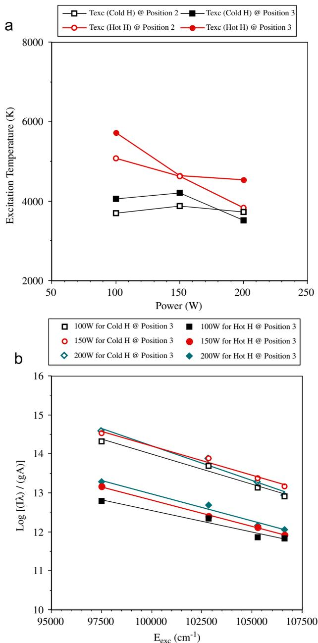
**Fig. 6 – (a) Excitation energy (Texc) determined as a function of power, position and hydrogen species used to determine peak intensity. (b) Boltzman plot showing the high fidelity of the data. Clearly computing excitation temperature on the ‘cold’ or ‘hot’ component of the line intensity makes only a small difference.**
