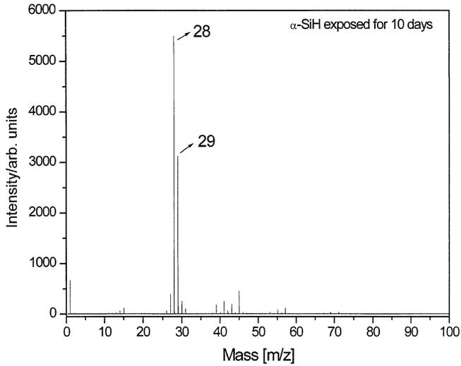
Fig. 4. The positive ion ToF-SIMS spectrum ( $m/e = 0-100$ ) of a nickel foil coated with an  $\alpha$ -SiH film and exposed to atmosphere for 10 days before the ToF-SIMS analysis that retained a large  $\text{SiH}^+$  peak.
