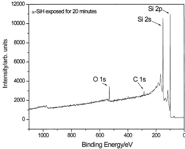
Fig. 12. The XPS survey scan of a nickel foil coated with an  $\alpha$ -SiH film and exposed to air for 20 min before XPS analysis showing minimal oxide and carbon.
