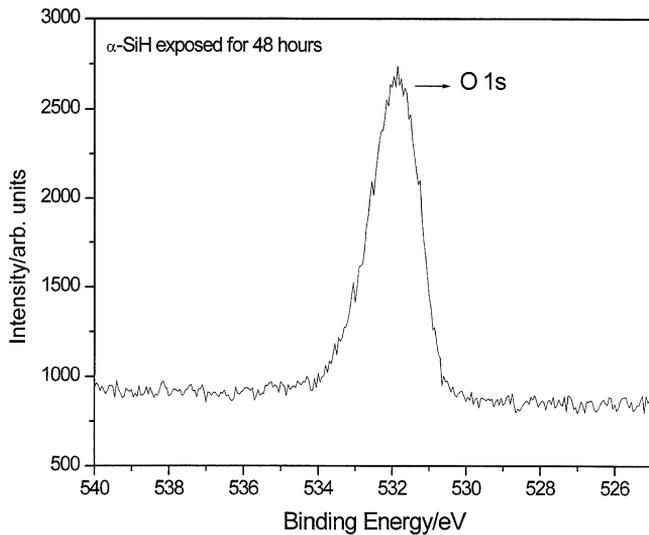
Fig. 17. The XPS spectrum (525–540 eV) in the region of the O 1s peak of a nickel foil coated with an  $\alpha$ -SiH film and exposed to air for 48 h before XPS analysis showing a minimal amount of oxide.
