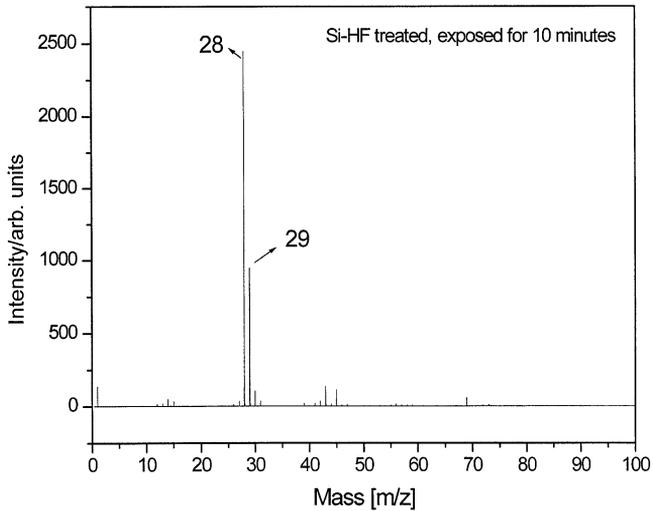
Fig. 5. The positive ion ToF-SIMS spectrum ( $m/e = 0-100$ ) of the HF cleaned silicon wafer exposed to air for 10 min before ToF-SIMS analysis.
