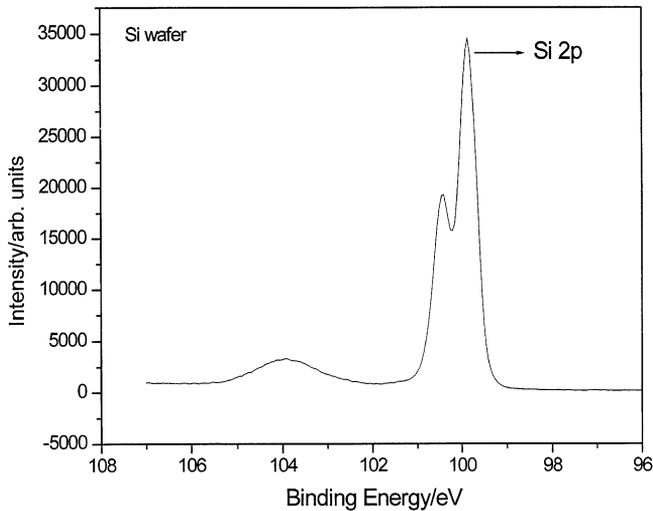
Fig. 13. The XPS spectrum (96–108 eV) in the region of the Si 2p peak of the noncoated cleaned commercial silicon wafer showing a large SiO<sub>2</sub> in the region of 104 eV.
