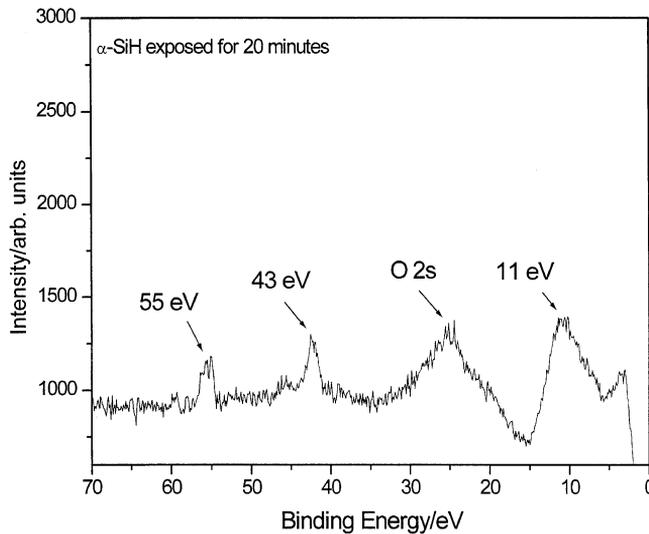
Fig. 21. The 0–70 eV binding energy region of a high-resolution XPS spectrum of a nickel foil coated with an  $\alpha$ -SiH film and exposed to air for 20 min before XPS analysis. The novel peaks observed at 11, 43 and 55 eV which could not be assigned to the elements identified by their primary XPS peaks matched and were assigned to highly stable silicon hydrides formed by the catalytic reaction of  $\text{He}^+$  and atomic hydrogen.
