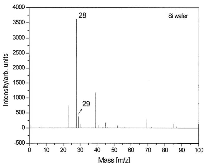
Fig. 2. The positive ion ToF-SIMS spectra ( $m/e = 0-100$ ) of a noncoated cleaned commercial silicon wafer (Alfa Aesar 99.9%).
