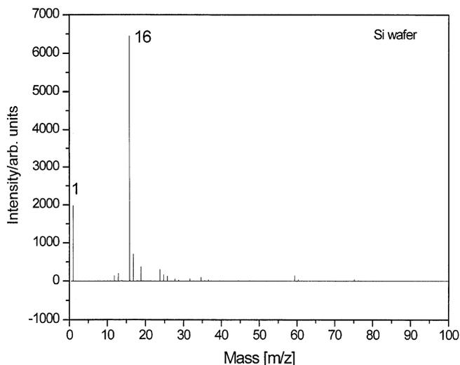
Fig. 6. The negative ion ToF-SIMS spectrum ( $m/e = 0-100$ ) of the noncoated cleaned commercial silicon wafer (Alfa Aesar 99.99%).
