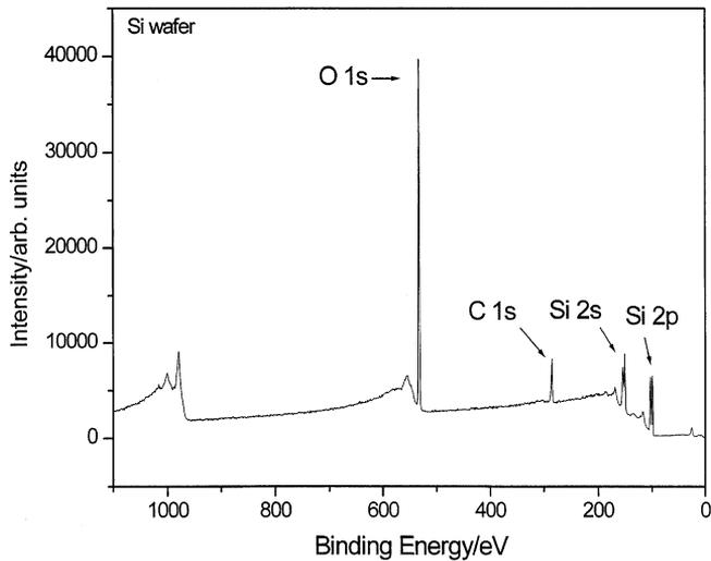
Fig. 11. The XPS survey scan of the noncoated cleaned commercial silicon wafer showing a large amount of oxide and carbon contamination of the surface.
