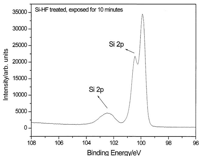
Fig. 16. The XPS spectrum (96–108 eV) in the region of the Si 2p peak of the HF cleaned silicon wafer exposed to air for 10 min before XPS analysis showing a very large SiO<sub>x</sub> peak in the region of 101.5–104 eV.
