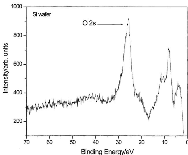
Fig. 19. The 0–70 eV binding energy region of a high resolution XPS spectrum of the commercial silicon wafer showing only a large O 2s peak in the low binding energy region.
