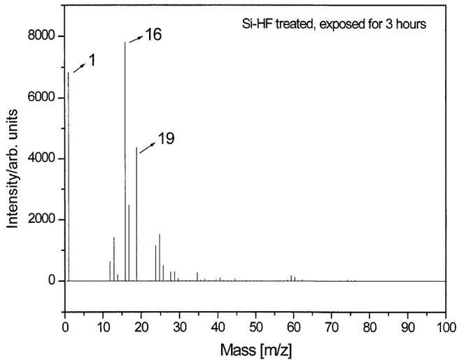
Fig. 10. The negative ion ToF-SIMS spectrum ( $m/e = 0-100$ ) of the HF cleaned silicon wafer exposed to air for 3 h before ToF-SIMS analysis showing a dominant oxide peak.
