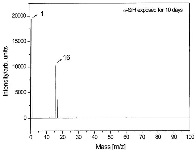
Fig. 8. The negative ion ToF-SIMS spectrum ( $m/e = 0-100$ ) of a nickel foil coated with an  $\alpha$ -SiH film and exposed to air for 10 days before the ToF-SIMS analysis that retained the dominant hydride ion peak.
