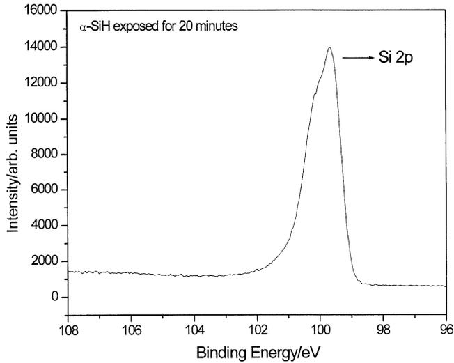
Fig. 14. The XPS spectrum (96–108 eV) in the region of the Si 2p peak of a nickel foil with an  $\alpha$ -SiH film and exposed to air for 20 min before XPS analysis showing no oxide in the region of 104 eV.
