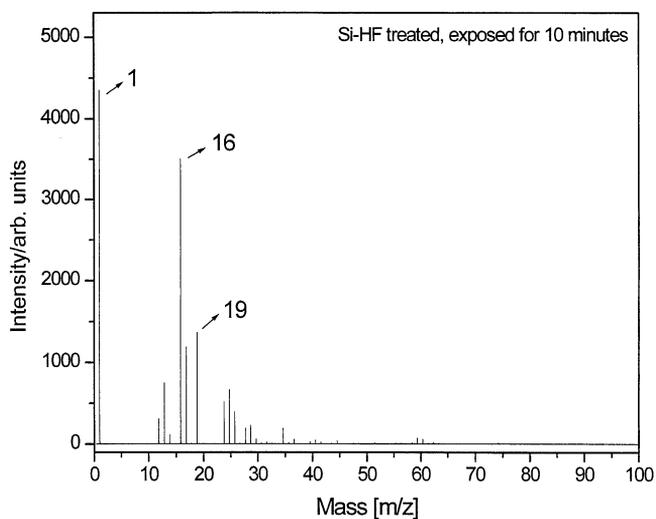
Fig. 9. The negative ion ToF-SIMS spectrum ( $m/e = 0-100$ ) of the HF cleaned silicon wafer exposed to air for 10 min before ToF-SIMS analysis.
