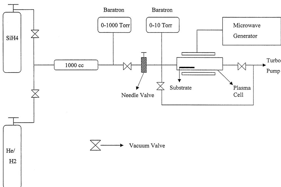
Fig. 1. The experimental set up comprising a microwave discharge cell operated under flow conditions.
