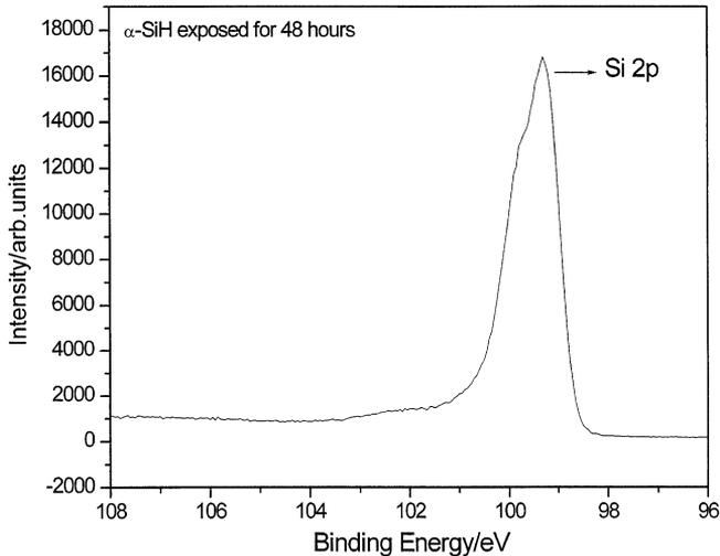
Fig. 15. The XPS spectrum (96–108 eV) in the region of the Si 2p peak of a nickel foil coated with an  $\alpha$ -SiH film and exposed to air for 48 h before the XPS analysis showing no oxide at 104 eV and possibly trace SiOH in the region of 102 eV.
