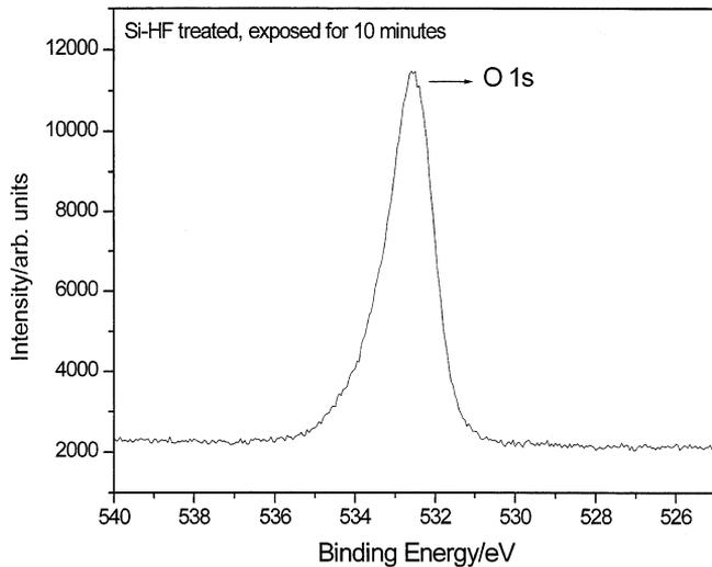
Fig. 18. The XPS spectrum (525–540 eV) in the region of the O 1s peak of the HF cleaned silicon wafer exposed to air for 10 min before XPS analysis showing a very large oxide peak.
