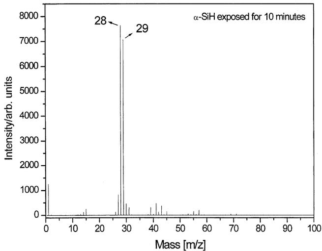
Fig. 3. The positive ion ToF-SIMS spectra ( $m/e = 0-100$ ) of a nickel foil coated with an  $\alpha$ -SiH film and exposed to air for 10 min that showed a large SiH<sup>+</sup> peak.
