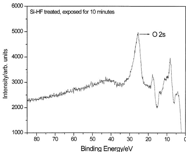
Fig. 20. The 0–85 eV binding energy region of a high resolution XPS spectrum of the HF cleaned silicon wafer exposed to air for 10 min before XPS analysis showing only a large O 2s peak in the low binding energy region.
