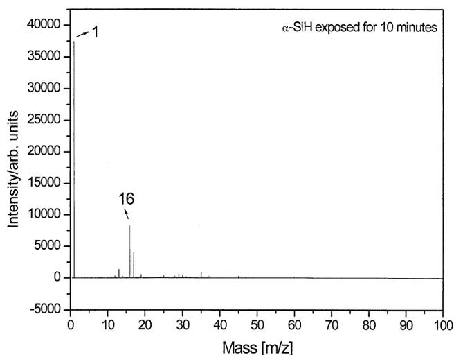
Fig. 7. The negative ion ToF-SIMS spectrum ( $m/e = 0-100$ ) of a nickel foil coated with an  $\alpha$ -SiH film and exposed to air for 10 min before ToF-SIMS analysis that was dominated by hydride ion.
